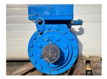
RIAL NUMBER S TRANE UA1L3871 HELIROTOR" COMPRESSOR MODEL NUMBER CHHPOM2TKDON092A ACO 50, 460 60-3 OCKED ROTOR CURRENT 50,246 60 LOCKED ROTOR CI 60 450. TILIZATION RAI 414-506 R134A
